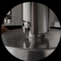
Tool attachment Easy self-locking bayonet
